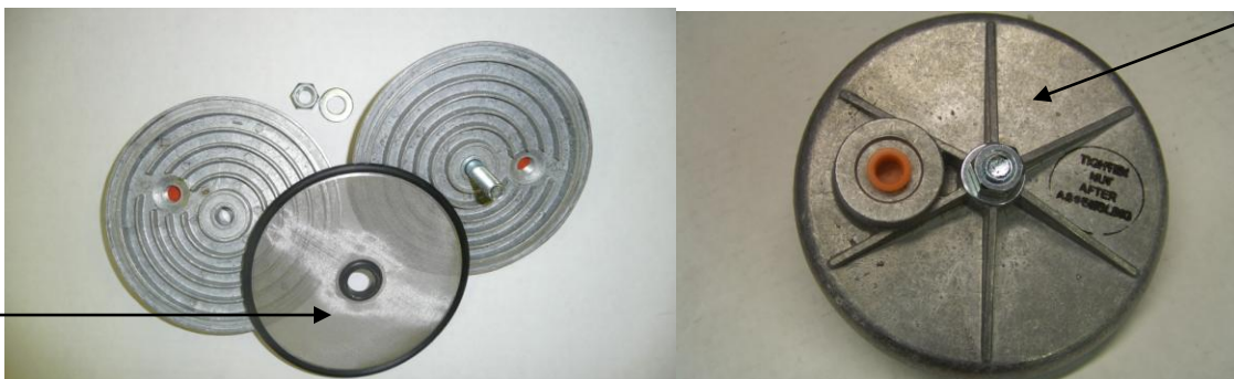
Figure 14 – Oil Filter (Spin-On Filter above, Pancake Style Filter below)
